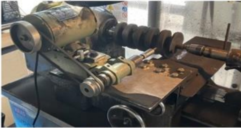
Custom CNC Mill/Lathe Constructed to Machine Graphite Screw Auger
