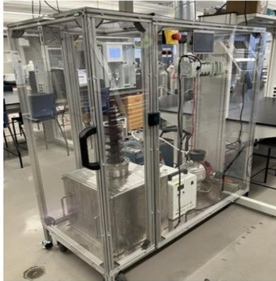
Partially Assembled Continuous Biochar Reactor
