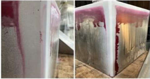
Dye Penetrant Welding Inspection Showing Passed (Right) and Failed (Left) Joints
