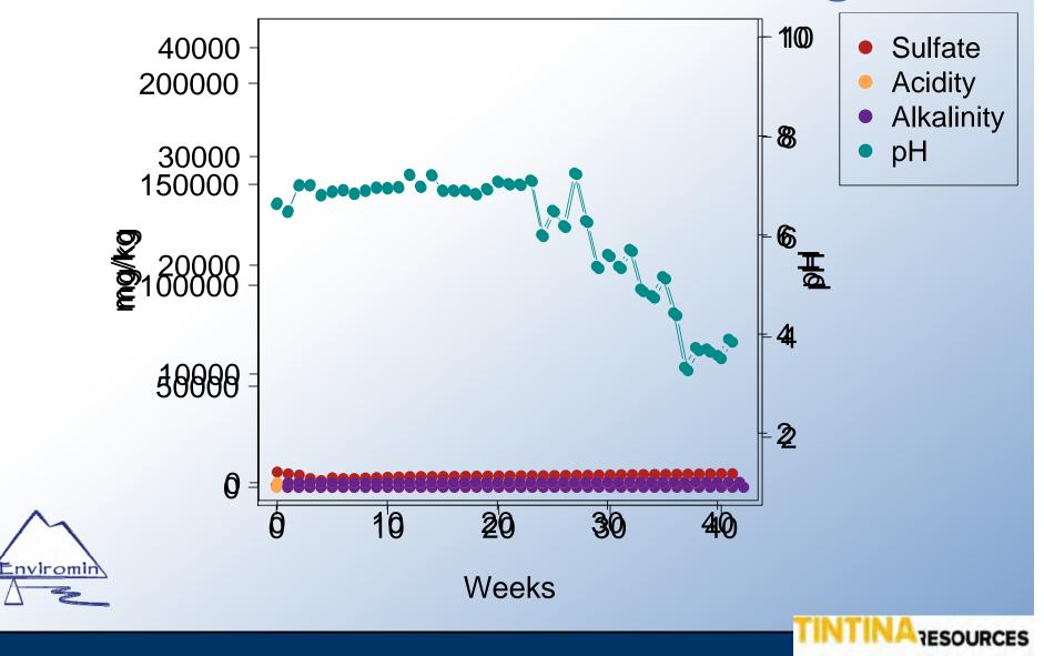
Details of Geochemical Tests
