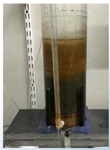
Conventional HCT test of flotation tailings (non-amended) under subaqueous conditions
