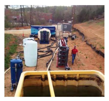
Electricity usage – Average **\$25.33/day-** includes 300 GPM CleanWave EC, Ultrafiltration, and all transfer pumps between equipment
