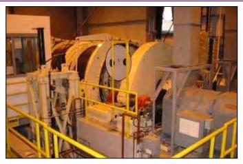
8' diameter Nordberg Hoist at Vent Shaft– 1400 Hp Mfg. 1954
