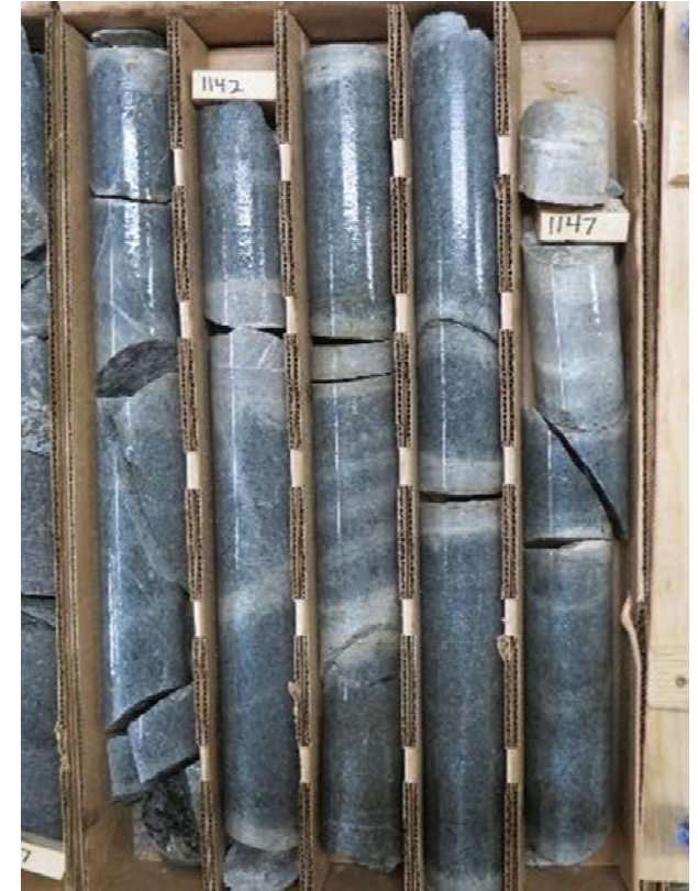
Latite porphyry showing propylitic alteration with phyllic alteration selvages around pyrite micro-veinlets
