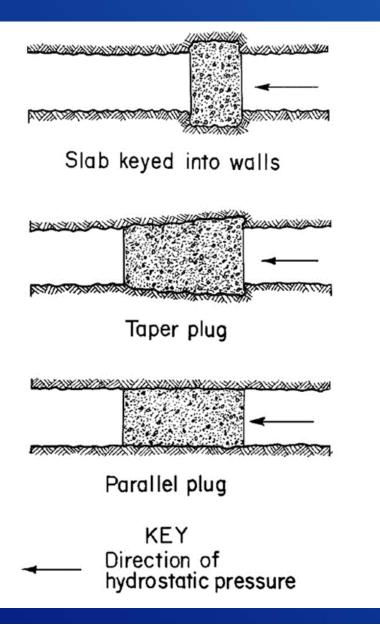
Heavily Reinforced, High Gradients, Extensive Grouting to Seal Plug
