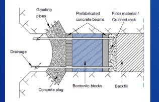
Combination concrete and soil plugs – clay with sand filters are being researched in Europe and Canada with hope to provide a long-term barrier after concrete fails
