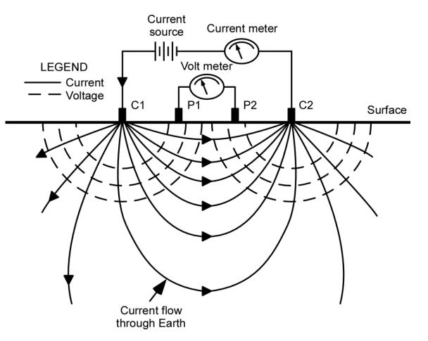
After ASTM D 6431: Standard Guide for using the direct current resistivity method for subsurface investigation
