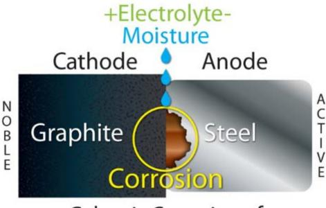
Galvanic Corrosion of Two Dissimilar Metals **Galvanic Series**
